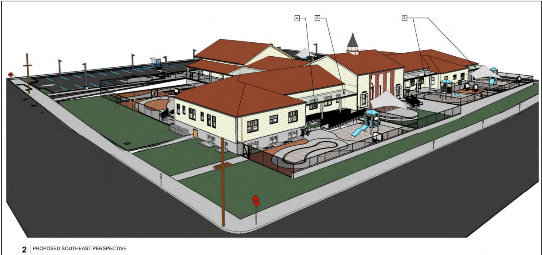
Figure 27 Proposed Southeast Perspective, with Mass/Scale and Colonial Revival-style Features Retained and Adapted for re-use as Childcare Center and Child Development Lab; Arrows Indicate Areas Slated for New Elements, Including Code-compliant Egress Doors, Windows, and Sun Canopies
