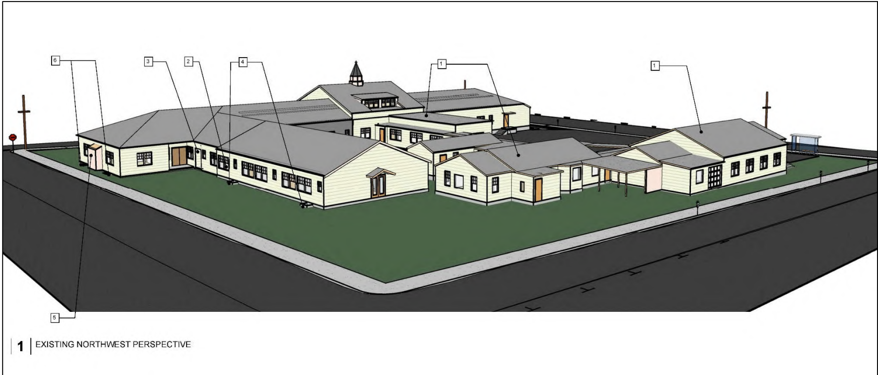
Figure 30 Existing Northwest Perspective, Showing Extant Rear Elevation and Additions over Time; Arrows Indicate Areas Slated for Limited Demolition/Removal and New Construction
