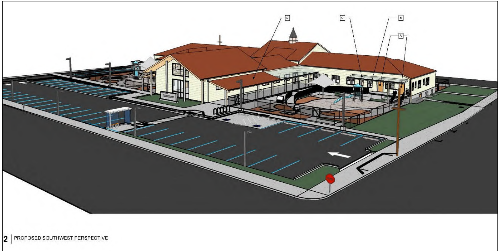
Figure 29 Proposed Southwest Perspective, Showing Proposed, More Compact Site Plan and Compatible New Construction; Arrows Indicate Areas Slated for New Elements, Including Code-compliant Egress Doors, Windows, and Sun Canopies
