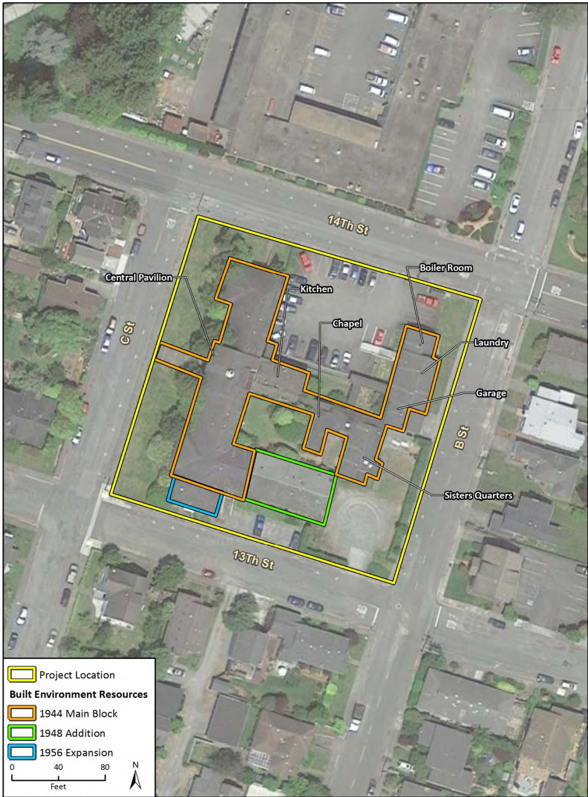
Figure 6 Trinity Annex, Building Components and Dates of Construction
