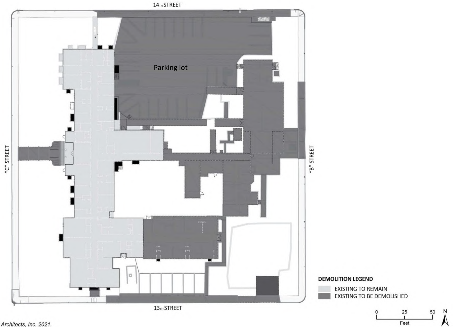
Figure 6 Demolition Site Plan
