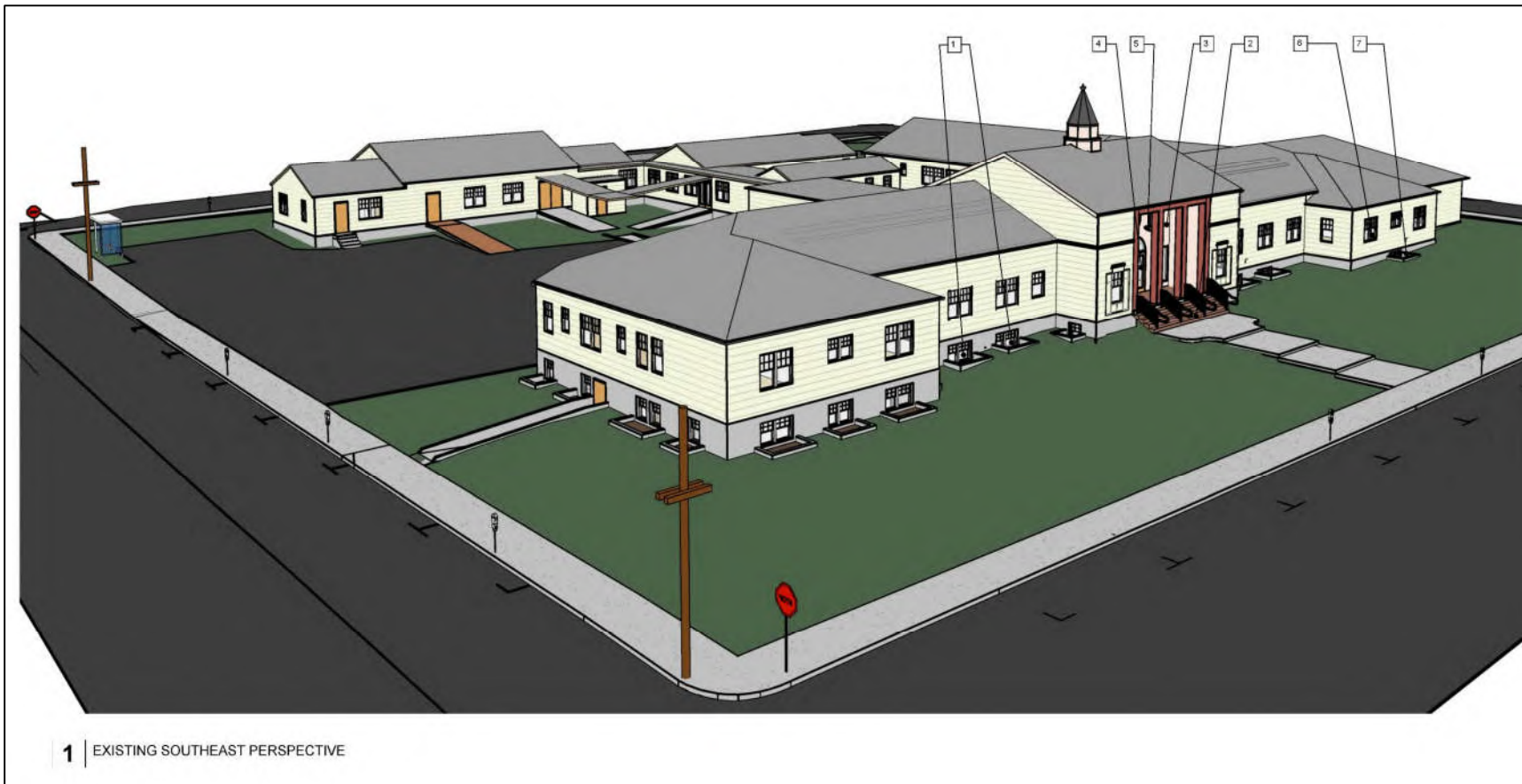
Figure 26 Existing Southeast Perspective, Showing Colonial Revival-style Features on Main Block Façade and Additions and Sheltered Breezeways on Rear Elevation; Arrows Indicate Areas Slated for Alteration, In-kind Replacement, Limited Demolition/Removal
