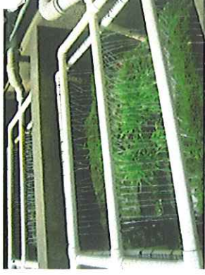
Biological filtration in the raceways
